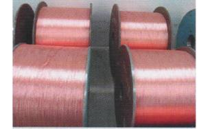
**Properties**: Multi-line drawing machines from Niehoff are used in the previous working procedure of bunching multi - line wires. As the diameters performance of products are consistence, the products possess the features of excellent flexibility, good performance, roundness, compactness and surface quality.
